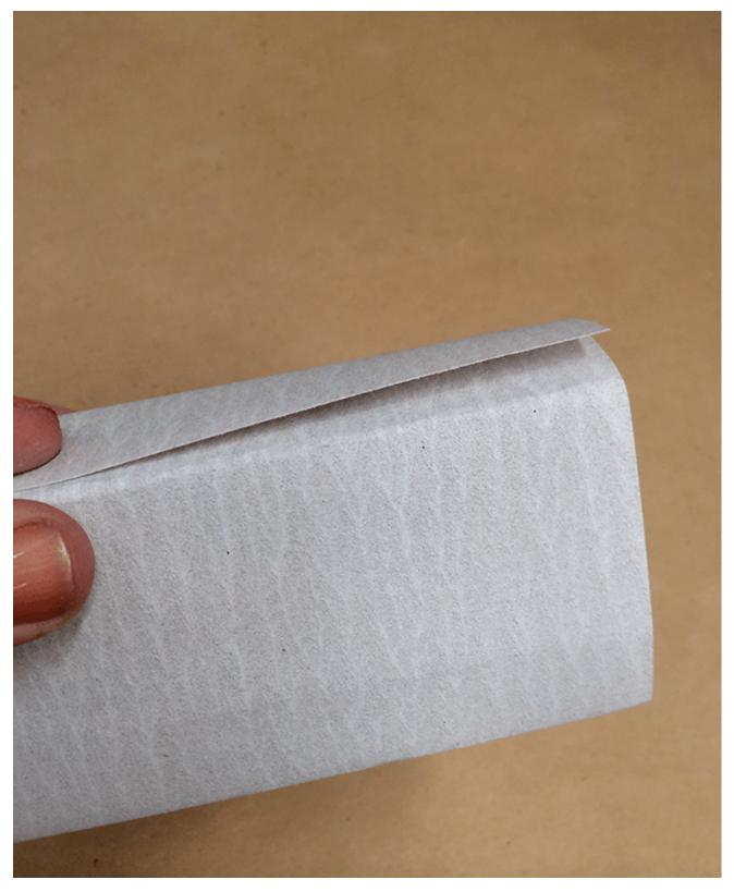
**5.** Hold the loose edge of the paper against the block while sanding. When the surfaces become smooth and worn, unfold the block to reveal the un-touched layer, refold and continue.
