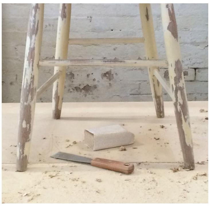
To makeover a basic timber chair you should use three grits of sandpaper, which is called abrasive paper by the pros, and a cork sanding block.
